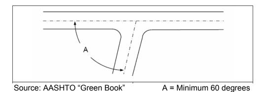
FIGURE 2-6 MINIMUM ANGLE OF INTERSECTIONS
