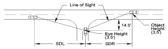
SDR = Sight Distance Right (For a vehicle making a left turn) SDL = Sight Distance Left (For a vehicle making a right or left turn)
