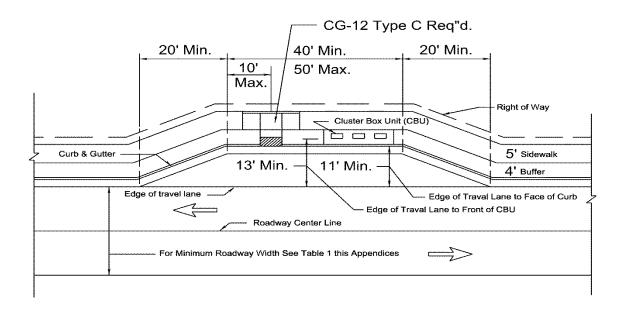
Detail for Cluster Box Unit Turnout - Curb & Gutter Typical Section\*
