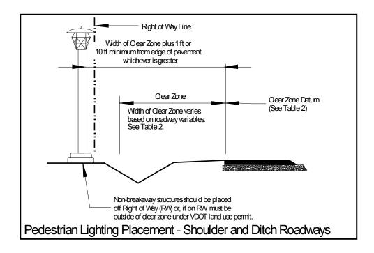
FIGURE 14 – LIGHTING ALONG SHOULDER AND DITCH SECTIONS
