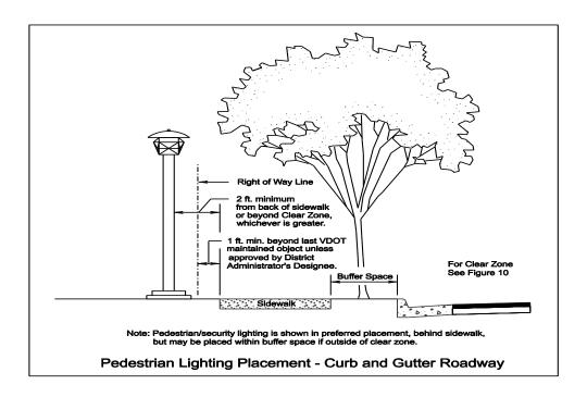
FIGURE 13 – LIGHTING ALONG CURB AND GUTTER SECTIONS\*
