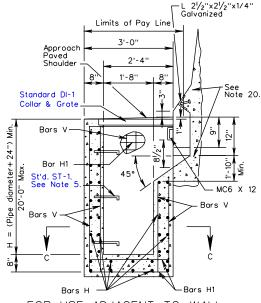
FOR USE ADJACENT TO WALL OR BARRIER WITH SAFETY SHAPE (TYPE II)
