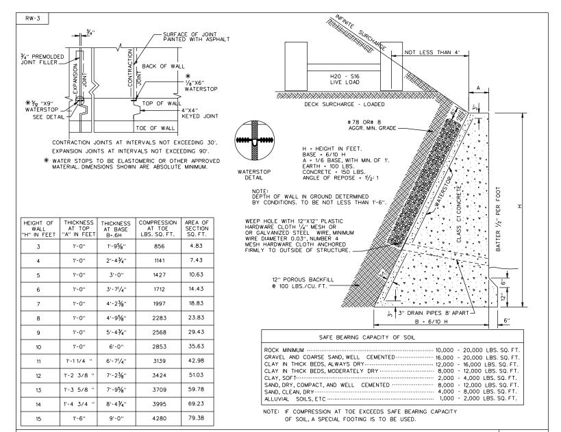
CONCRETE GRAVITY RETAINING WALLS
