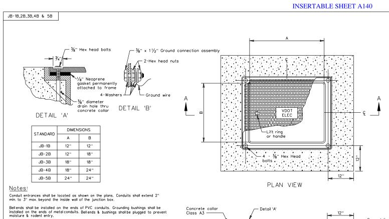
\*Depth of conduit entrances for magnetic detectors shall be in accordance with Standard TD-2.
