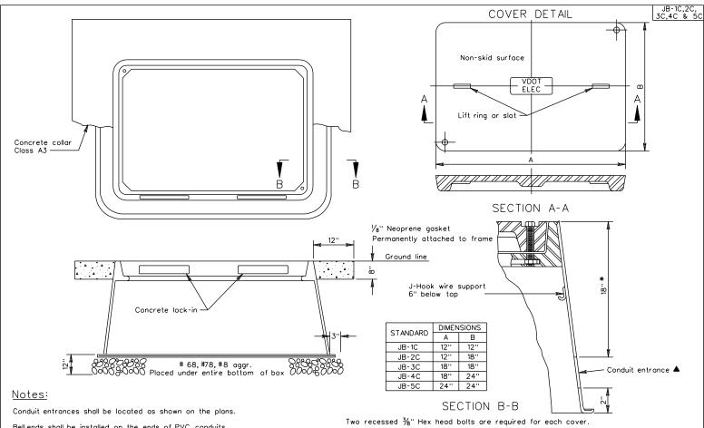
Bell ends shall be installed on the ends of PVC conduits. Grounding bushings shall be installed on the ends of metal conduits. Bell ends and bushings shall be plugged to prevent moisture and rodent entry.
