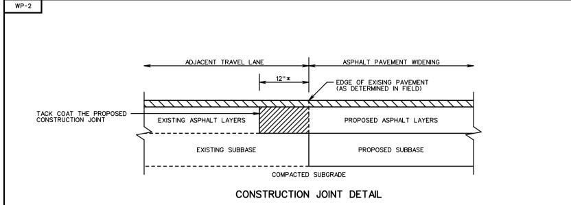
REMOVE EXISTING ASPHALT LAYERS TO EXISTING SUBBASE AND REPLACE WITH PROPOSED ASPHALT WIDENING LAYERS
