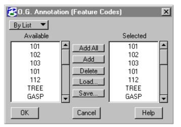
This dialog box is activated when the Select Feature Codes option button of the Design Section Display dialog box is clicked. It allows for the annotation of selected featured coded original cross section points retrieved from the DTM.
