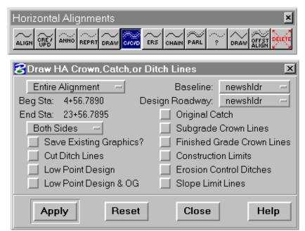
This command displays in the horizontal view, the crown, catch, and ditch point lines of a roadway from the IGrds Working files. (Straight lines are drawn between design cross sections.)
