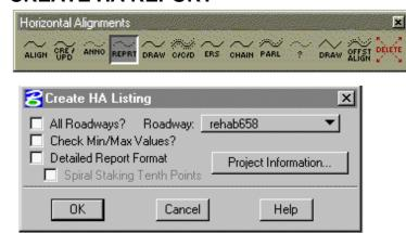
This command creates a horizontal alignment listing in the temporary report file (.tmp) for the specified roadway(s).
