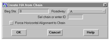
This command creates a new horizontal alignment which coincides with a previously stored geometry chain or MicroStation Chain/ Smartline.
