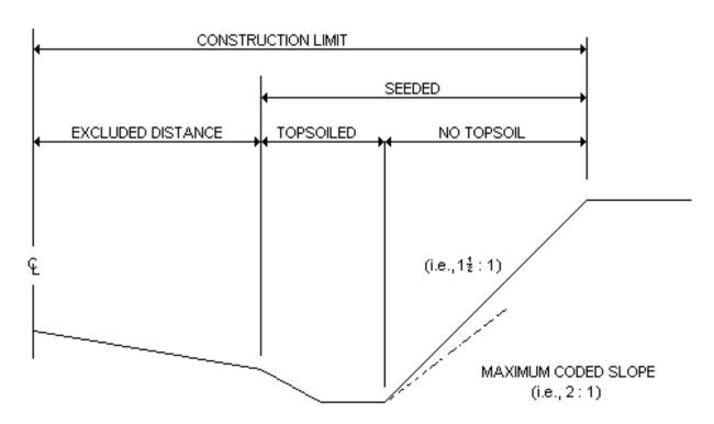
The topsoil placement volumes computed are the amounts needed to cover the areas disturbed by construction from a specified distance left and right of the roadway centerline to the slope stake. The topsoil depth and maximum slope ratio for placing topsoil are required input. The seeding areas are for all slopes from a specified distance left and right of the roadway centerline to the slope stake.
