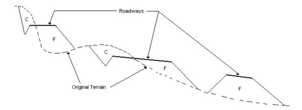
These end areas are maintained in the cross section file for the appropriate baseline until the design is changed. They are available for volume computations using any combination of design roadways associated with the baseline. The volume computations are made by roadway between each terrain cross section and quantities thus computed are accumulated by roadway. This process provides considerable versatility in analyzing quantities.
