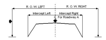
Right-of-way width left is on the RIGHT side of terrain centerline
