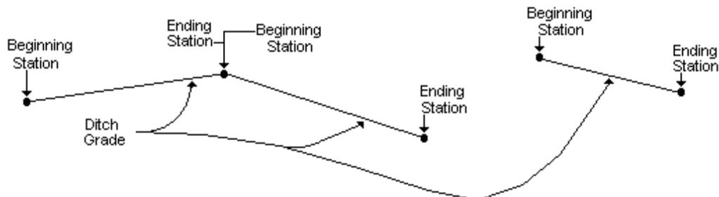
The grade line type special ditches need not be continuous.
