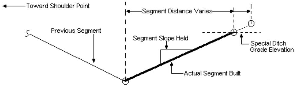
Figure I-1a - S Special Ditch Option, Grade Line Type Special Ditch
