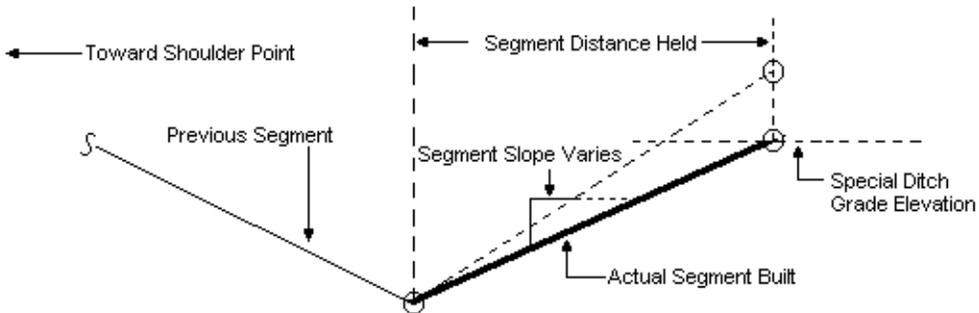
Figure I-2a - D Special Ditch Option, Grade Line Type Special Ditch
