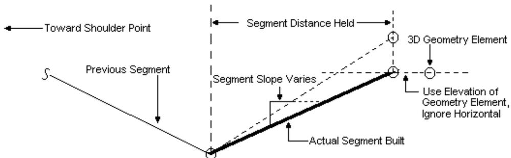
Figure I-2b - D Special Ditch Option, 3D Geometry Element Type Special Ditch
