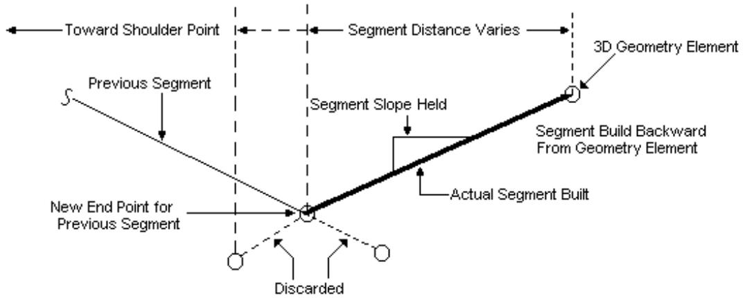
Figure I-3 - T Special Ditch Option
