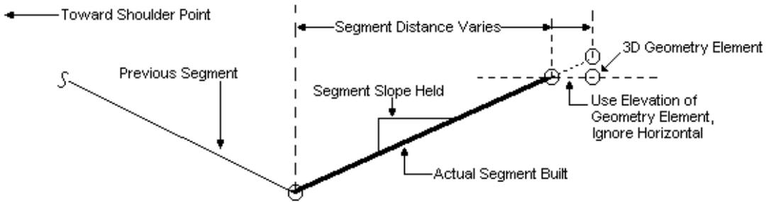
Figure I-1b - S Special Ditch Option, 3D Geometry Element Type Special Ditch
