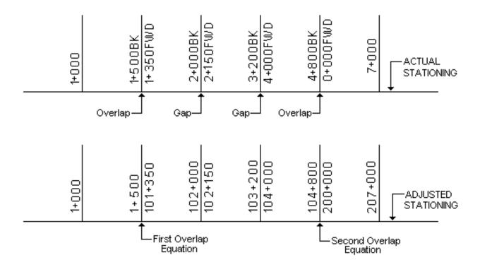
Figure A-2 - Examples of Equation Numbering and Stationing Scheme - Metric Units
