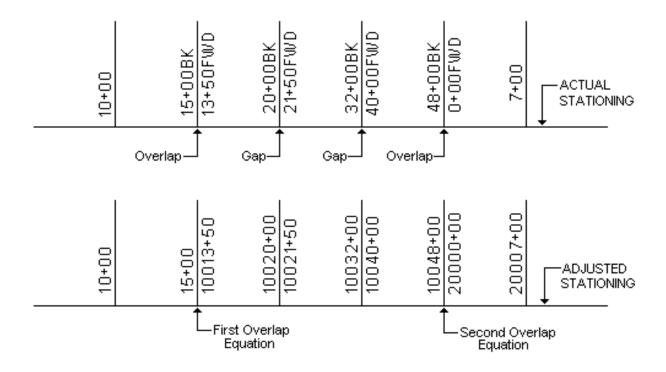
Figure A-1 - Examples of Equation Numbering and Stationing Scheme - Imperial Units
