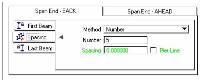
The screenshot shows the 'Beam Group Specifications' dialog box with the 'Spacing' tab selected. The 'Span End - BACK' and 'Span End - AHEAD' tabs are visible at the top. The 'Method' dropdown is set to 'Number'. The 'Number' field contains '5'. The 'Spacing' field contains '0.000000'. The 'Pier Line' checkbox is unchecked.
