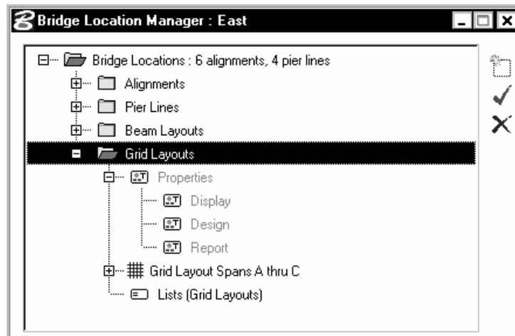
*Grid Layout Spans A thru C shown*
