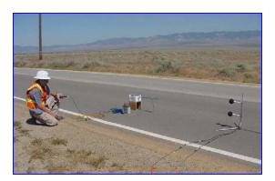
Trial adjustment of tire/pavement source noise using OBSI data
