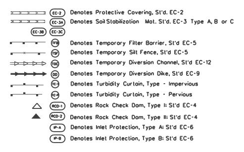
The ESC symbols are to be used to denote proposed erosion and sediment control items on the plans and are available in the CADD Cell and Custom Line Style Libraries and the GeoPak Road Plan View Labels.
