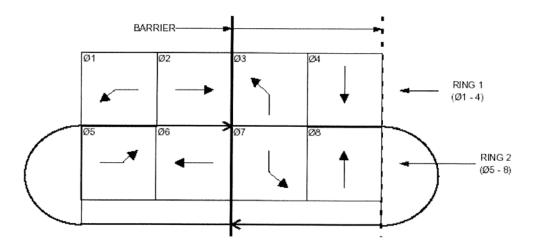
Figure 2-4: NEMA - DUAL RING CONFIGURATION
