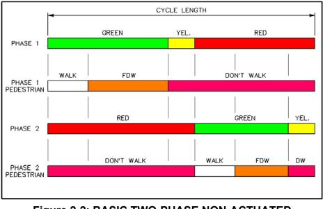
Figure 2-2: BASIC TWO-PHASE NON-ACTUATED OPERATION WITH PEDESTRIAN INTERVALS
