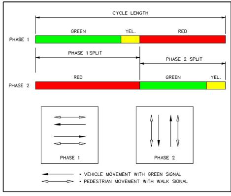
Figure 2-1: BASIC TWO-PHASE NON-ACTUATED OPERATION
