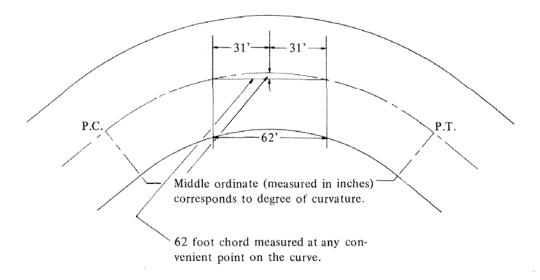
Central angle may be determined by multiplying the length of the curve from P.C. (beginning of curve) to the P.T. (end of curve) by the degree of curvature (as found above) and divide that product by 100'.
