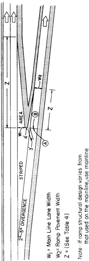
that used on the mainline, use mainline design on (A) side of separation line and Ramp design on (B) side.
