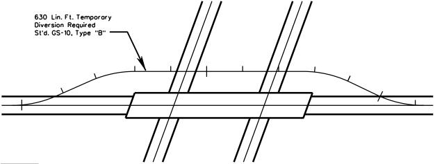
Detours on crossroads carrying over 750 ADT should have the complete alignment, grades, typical sections, drainage, etc., shown on the plans. Additional temporary construction easement lines should also be shown, if necessary.
