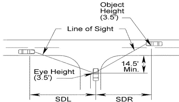
SDR = Sight Distance Right (For a vehicle making a left turn)
