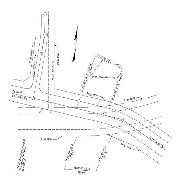
FIGURE C-3-1 SKETCH SHOWING SURVEY PROPERTY LINE TIE AND PROPOSED R/W BREAK POINT\*
