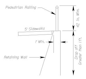
Railing is required when sidewalk is constructed adjacent to a vertical drop-off greater than 1'. However, gripping rail is required <u>only</u> when the slope of the sidewalk is 5% or greater. Contact the Location and Design Standards and Special Design Section for details.
