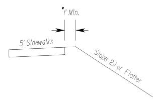
\* No railing is required if a 1' min. graded area is provided at the back of sidewalk when the slope is 2:1 or flatter, unless adjacent to a parallel water hazard 2' deep or other obvious hazard. If a railing is required the graded area behind the sidewalk shall be increased by 1' to accommodate the railing. Contact the Location and Design Standards and Special Design Section for details.
