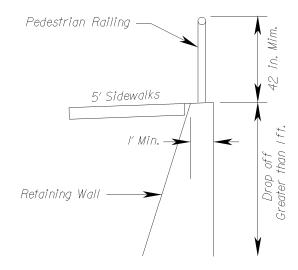
Railing is required when sidewalk is constructed adjacent to a vertical drop-off greater than 1'. However, gripping rail is required <u>only</u> when the grade of the sidewalk is 5% or greater. Contact the Location and Design Standards and Special Design Section for details.
