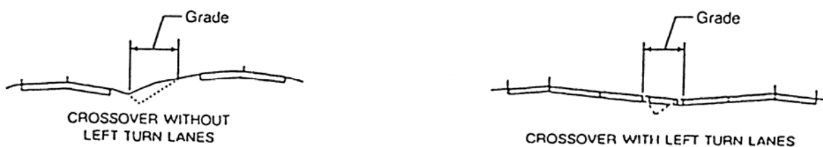
Determination of Grade on a Crossover
