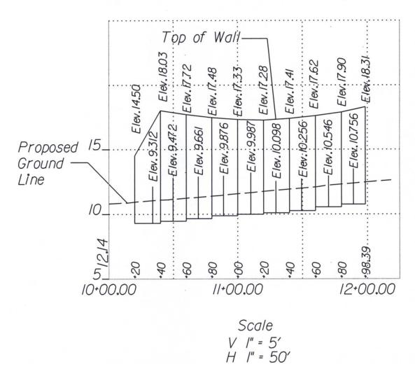
FIGURE 2E-8 PROFILE FOR PROPOSED RETAINING WALL
