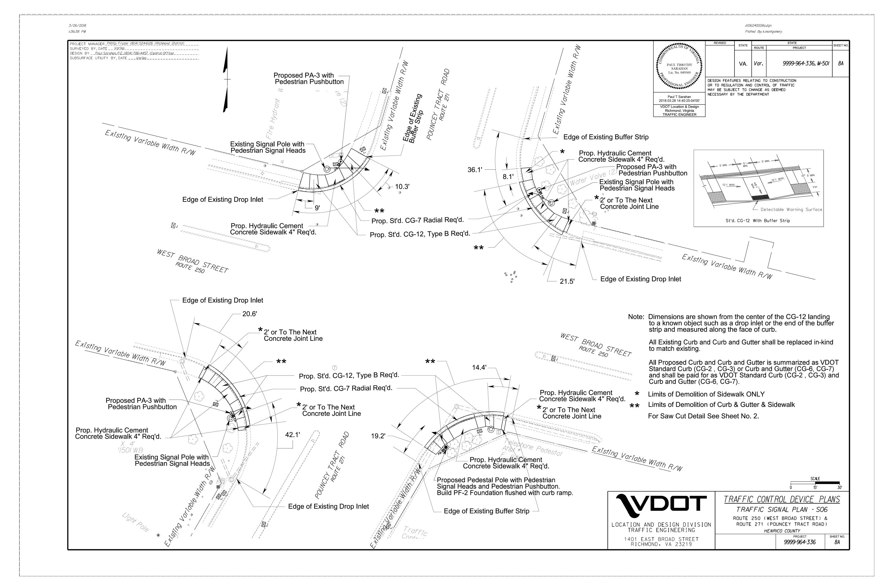
FIGURE 2H - 42 SAMPLE PEDESTRIAN CROSSWALK PLAN (FOR ALTERATION PROJECTS ONLY)
