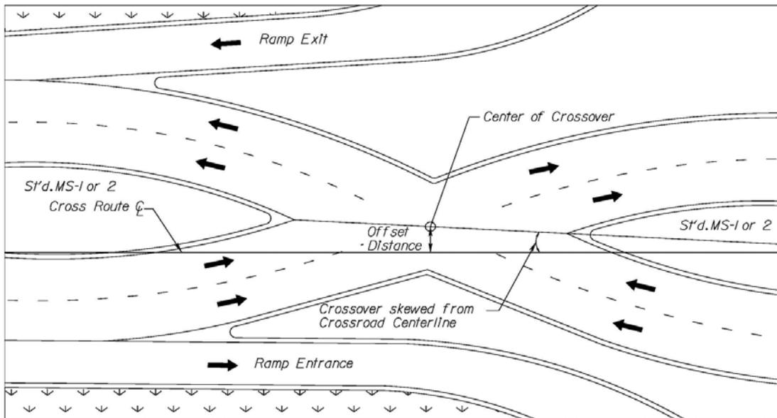
**FIGURE A-3-5 OFFSET DISTANCE FOR INTERSECTION**
