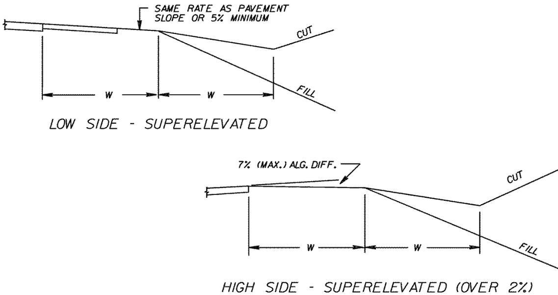
NOTE: FOR WIDTH OF SHOULDERS AND DITCHES (W) SEE GEOMETRIC DESIGN STANDARDS.
