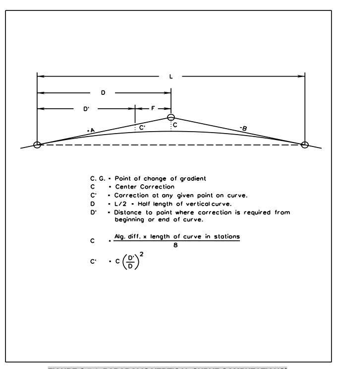
FIGURE C-7-6 PARABOLIC VERTICAL CURVE COMPUTATIONS\*
