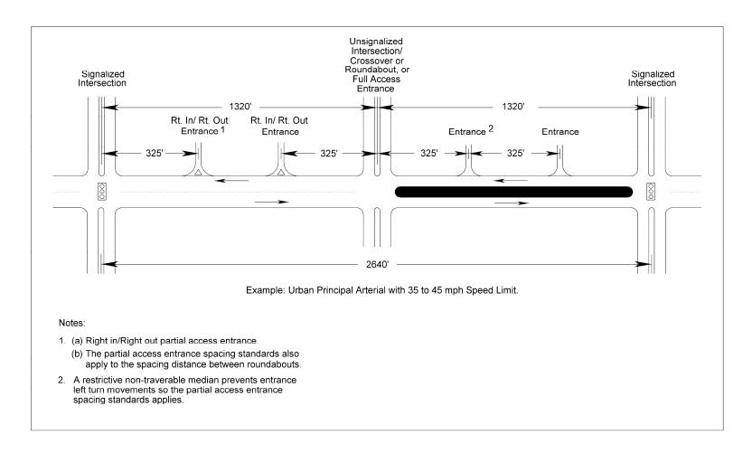
FIGURE 2-8.1 ILLUSTRATION OF THE RELATIONSHIP BETWEEN SPACING STANDARDS\*
