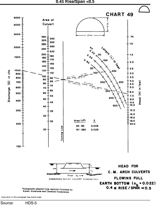
Appendix 8C-49 Outlet Control, Corrugated Metal Arch, Earth Bottom, 0.4≤ Rise/Span <0.5
