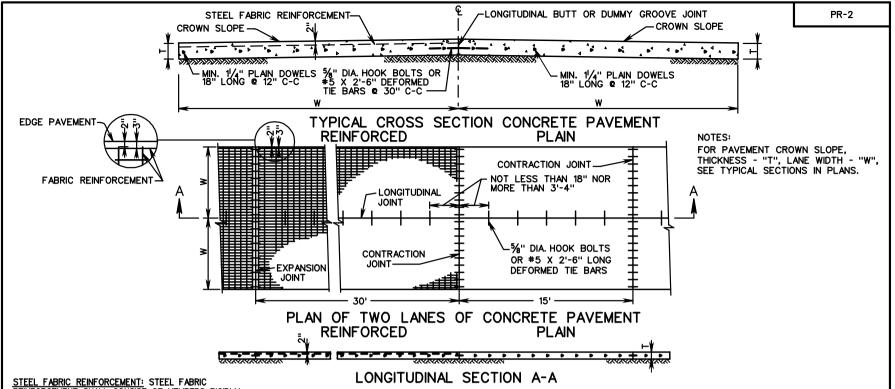
REINFORCEMENT SHALL CONSIST OF MEMBERS RIGIDLY ATTACHED AT ALL JOINTS OR POINTS OF INTERSECTION EXCEPT AS NOTED BELOW:(\*). LONGITUDINAL MEMBERS SHALL BE OF NO. 2 GAGE WIRE SPACED AT 6" ON CENTERS. TRAVERSE MEMBERS SHALL BE NO. 4 GAGE WIRE, SPACED AT 12" ON CENTERS. (WIRE REINFORCEMENT STEEL INSTITUTE DESIGNATION 6 X 12 - W5.5 X W4).
