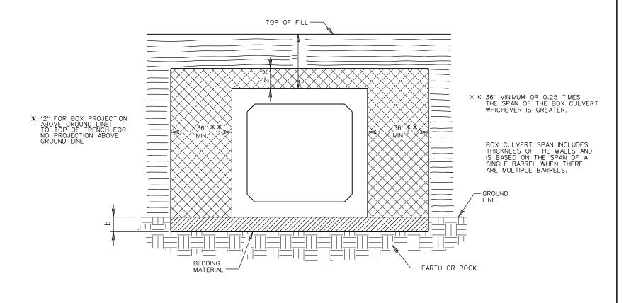
H = HEIGHT OF COVER MEASURED FROM TOP OF CULVERT TO FINISHED GRADE.
