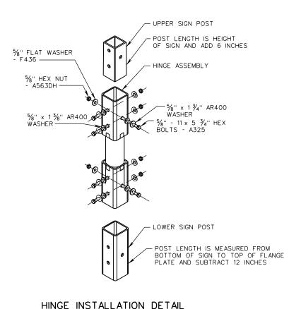
1. HINGE ASSEMBLY SHALL BE USED FOR MULTI-POST
