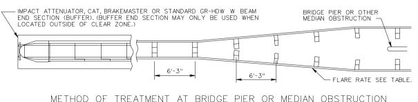
BLOCKED-OUT W BEAM MEDIAN BARRIER
