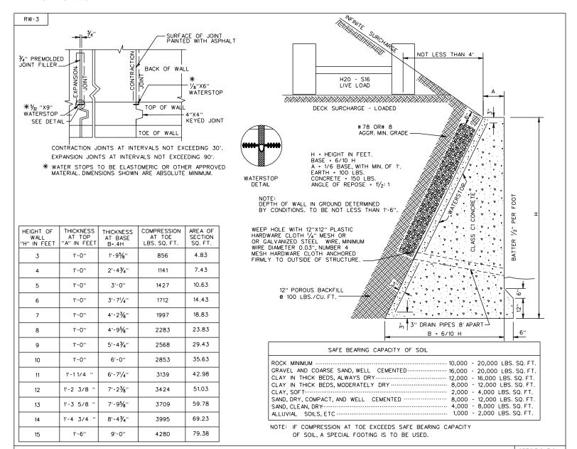
CONCRETE GRAVITY RETAINING WALLS
