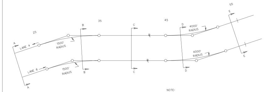
WHEN  $\mbox{\ensuremath{\mathbb{Q}}}$  (CROWNLINE) IS ON THE INSIDE EDGE OF PAVEMENT, TANGENT SECTIONS ARE TO BE CODED AS STRAIGHT.
