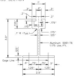
TYPICAL DETAILS FOR TYPE VA SIGN STRUCTURES
