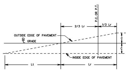
SUPERELEVATED BY AN AMOUNT EQUAL TO THE STANDARD PAVEMENT CROWN
