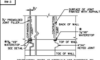
CONTRACTION JOINTS AT INTERVALS NOT EXCEEDING 30'. EXPANSION JOINTS AT INTERVALS NOT EXCEEDING 90'.
