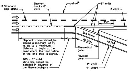
\* The pavement marking for the mainline of Interstate Highways shall be 6" wide; all other highways the pavement marking shall be 4" wide unless otherwise noted on the plans.
