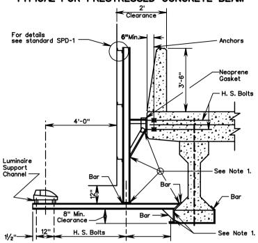
This parapet is not typical for bridges with a sidewalk. Bridge plans shall be reviewed for project specific parapet/rail.
