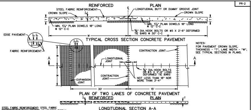
STEEL FABRIC REINFORCEMENT: STEEL FABRIC REINFORCEMENT SHALL CONSIST OF MEMBERS RIGIDLY ATTACHED AT ALL JOINTS OR POINTS OF INTERSECTION EXCEPT AS NOTED BELOW:(\*). LONGITUDINAL MEMBERS SHALL BE OF NO. 2 GAGE WIRE SPACED AT 6" ON CENTERS. TRAVERSE MEMBERS SHALL BE NO. 4 GAGE WIRE, SPACED AT 12" ON CENTERS. (WIRE REINFORCEMENT STEEL INSTITUTE DESIGNATION 6 X 12 - W5.5 X W4).
