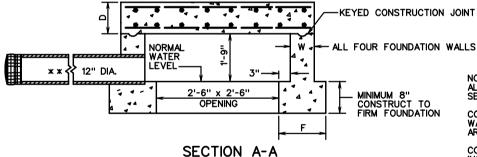
ALL CONCRETE TO BE CLASS A3 IF CAST IN PLACE. FOR PRECAST SEE SHEET 110.02.
