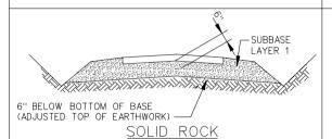
REMOVE ROCK TO A POINT 6" BELOW BOTTOM OF BASE FOR ENTIRE WIDTH OF ROADWAY. BACKFILL WITH SUBBASE LAYER 1 USING BOTTOM 2" AS A LEVELING COURSE.
