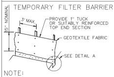
SUPPORTS FOR TEMPORARY FILTER BARRIERS SHALL BE A NOMINAL 1" X 2" OR A 1½" DIA. NO. 2 SOUTHERN PINE OR OAK, OR STEEL HAVING A MIN. WEIGHT OF 1.00 LBS. PER LINEAR FOOT.
