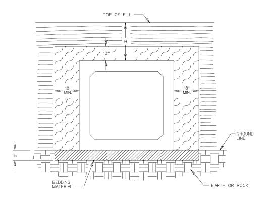
H = HEIGHT OF COVER MEASURED FROM TOP OF CULVERT TO FINISHED GRADE.
