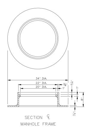
NOTES: STRUCTURAL COMPONENTS SHALL CONFORM TO AASHTO M222.
