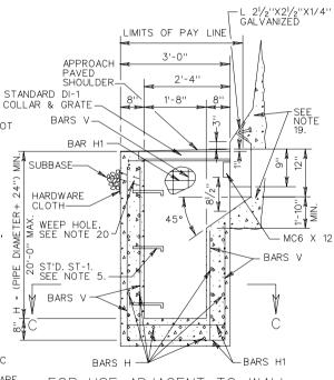
FOR USE ADJACENT TO WALL OR BARRIER WITH SAFETY SHAPE (TYPE III)
