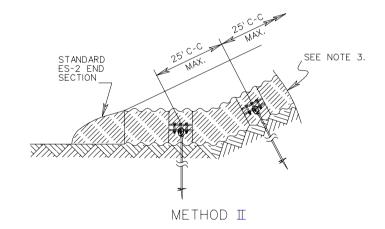
METHOD OF OUTLET PIPE INSTALLATION FOR DI-13
