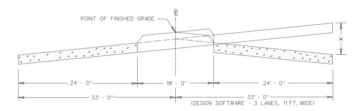
\* THE ELEVATION DIFFERENTIAL BETWEEN NORMAL CROWN AND MAXIMUM SUPERELEVATION, RELATIVE TO THE BASELINE PROFILE.
